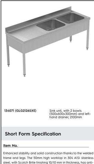
steel, with Scotch Brite finishing 10/10 mm in thickness, has antidrip edges, welded corners and overflow rim along the top. 2 welded and polish sink bowls in 304 AISI stainless steel supplied with overflow pipe and 2" drain hole. Upstand h=100mm with 10mm radius corner covered on the back with AISI 304 stainless steel spot welded profile. Square section legs and height adjustable feet (-20/+30 mm) in 304 AISI stainless steel.
